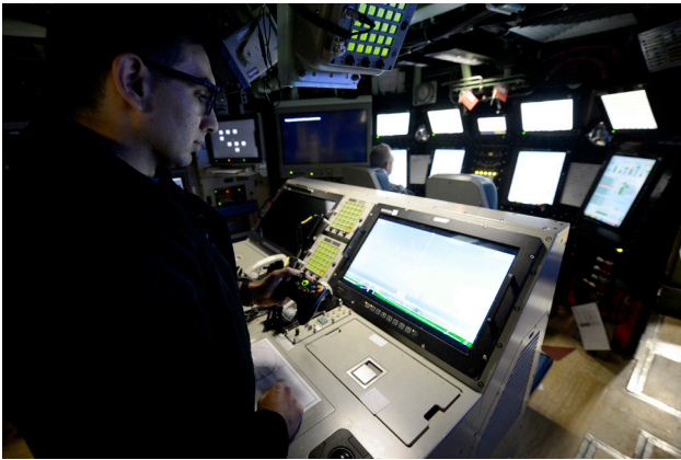
PORT CANAVERAL, Fla., (January 12, 2018) Lt. Anthony Matus uses an Xbox controller to maneuver the photonic mast
